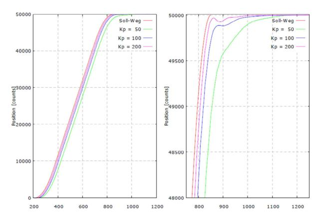
It can be observed, that a following error is occurring. The higher the Kp value of the controller the smaller the following error is. If the Kp value is too high, an overshoot can occur. This will also happen if the acceleration or deceleration is too high (> 10ms/1000rpm).
