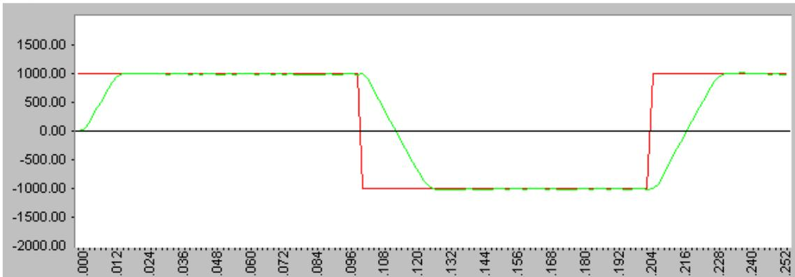
Amplifier tuning for 5.04x $J_m$  load. L.I. =432%, BW. = 90Hz., T.F. = 130
