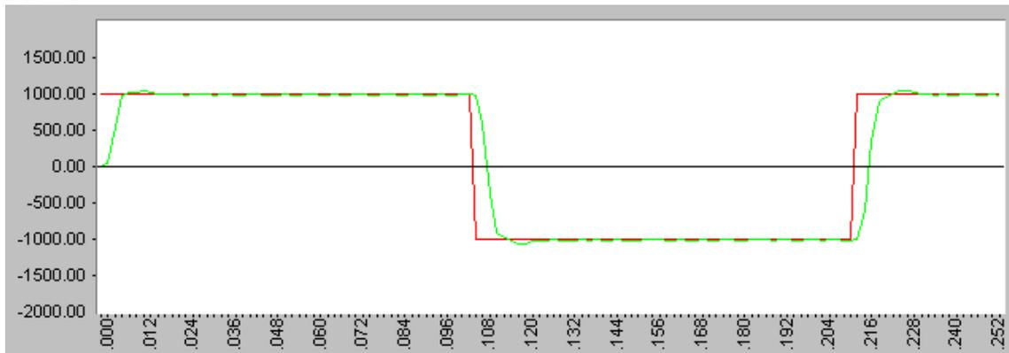
Pole placement tuning for  $J_m$  only. Amplifier tuning parameters: L.I. = 1%, BW. = 90Hz., T.F. = 100 (overshoot = 1050 rpm)
